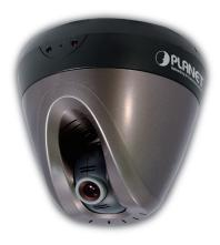
Equipped with Pan & Tilt functions, the PLANET ICA-501 is a CCD PT Internet Camera which offers pan range of 355-degree and tilt range of 100-degree with high-speed controlling (Pan:180 degree/sec, Tilt:100 degree/sec) over Ethernet. Expect the indoor installation, the optional outdoor housing of PLANET ICA-OH is perfect to expand users applications where users may combine the ICA-501 to enhance the flexibility of internet surveillance.
